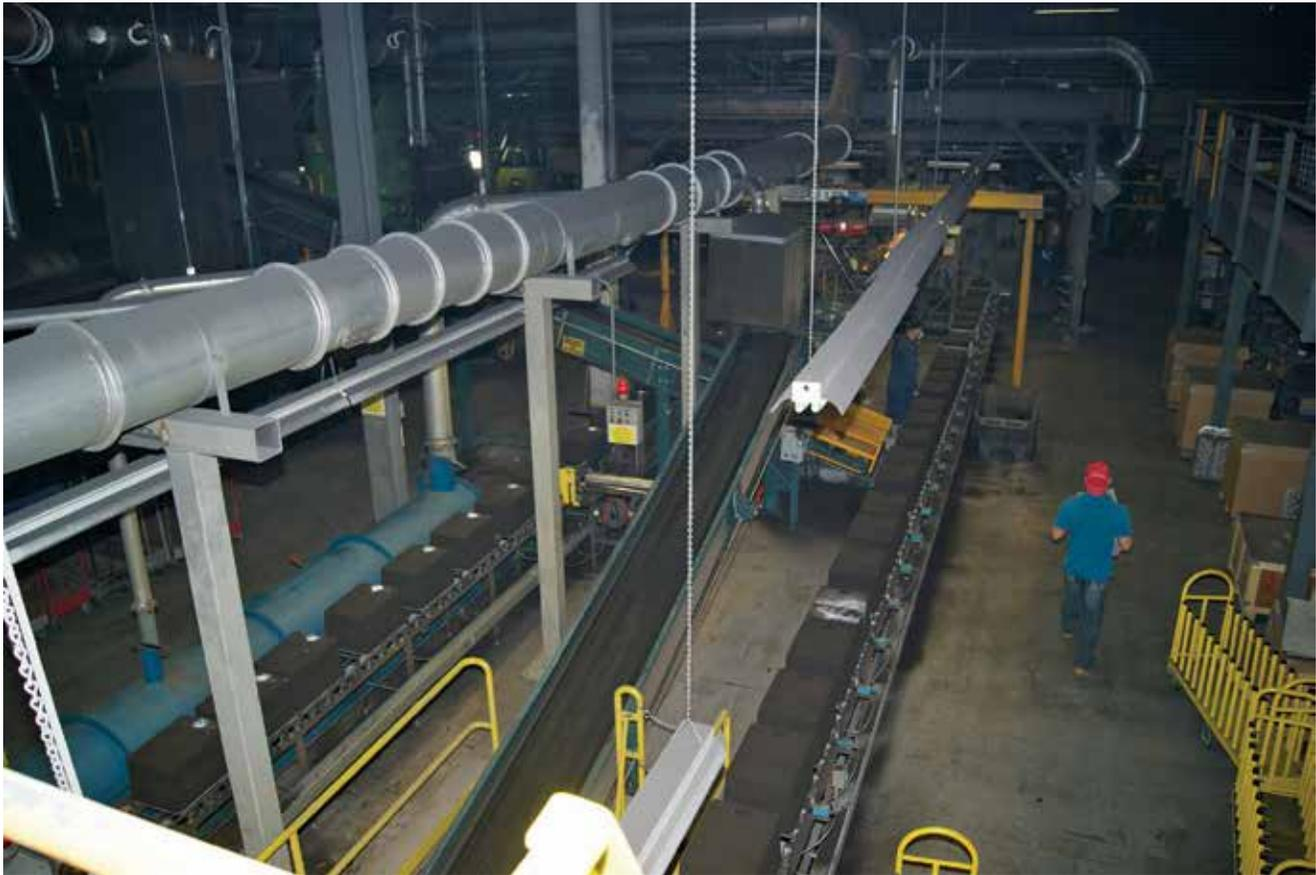
Richmond Industries uses two molding lines to pour aluminum and copper-based castings, including this Hunter automated matchplate molding line.
