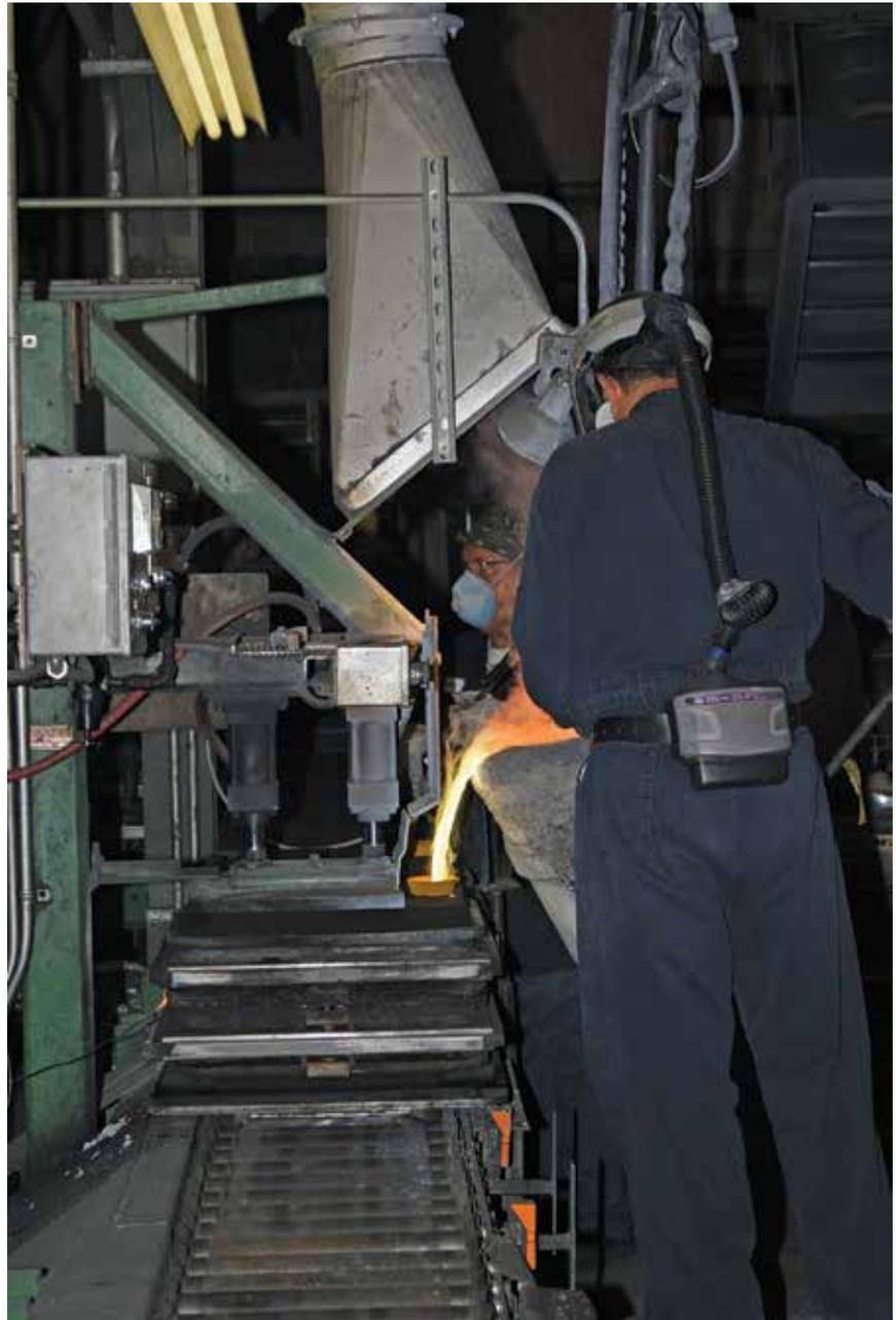
The metalcasting facility mainly pours two aluminum alloys and a dozen copper-base alloys, but offers other options depending on customer need. The facility also pours lead-free alloys.
